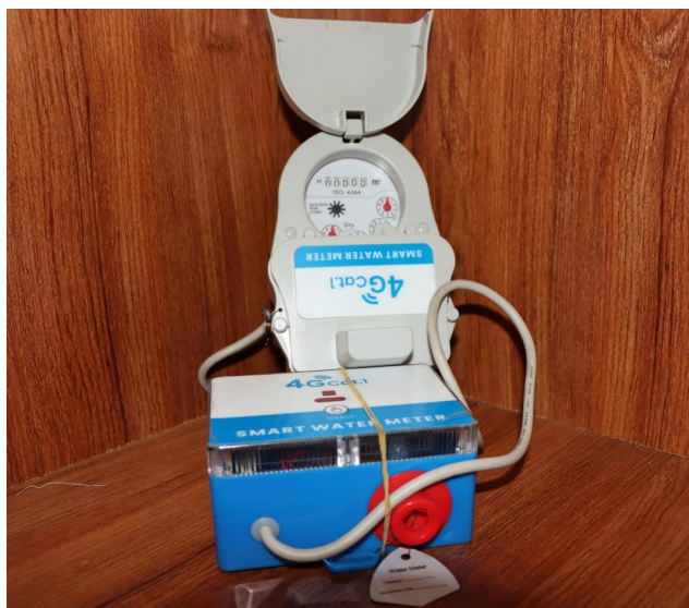
A smart water meter on display at KEWI Non-Revenue Centre of Excellence laboratory.
