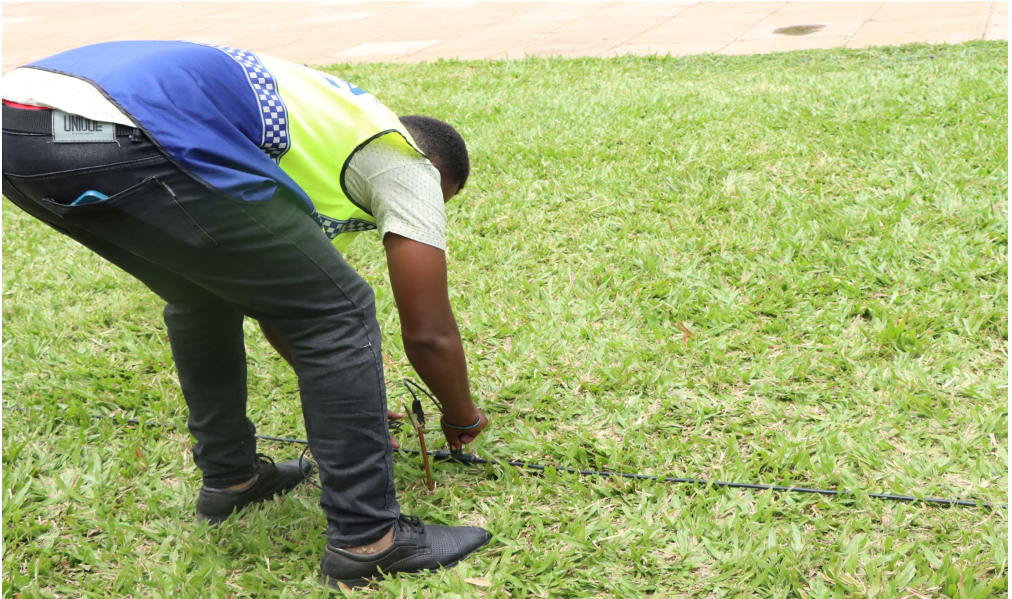
A student demonstrates how electrodes are driven into the ground and connected to the main unit of the detector. Hydro-geophysical surveys are essential not just for finding water, but also for geotechnical purposes.
